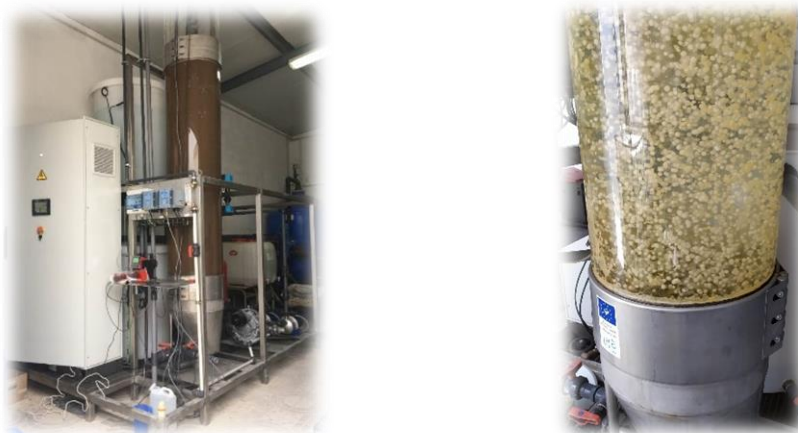
Figure 13: Bioreactor 1 after inoculation with activated sludge (left) and after start-up with denitrifying granules (right).
