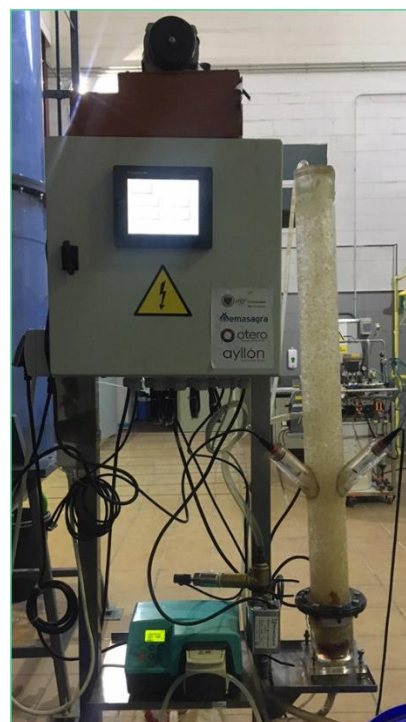
Figure 5. Cylindrical bioreactor treating polluted groundwater in sequential stages.
