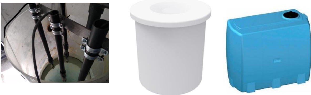
Figure 9: Detail of the probes and measuring systems (left), buffer tank (centre) and nutrient tank (right).
